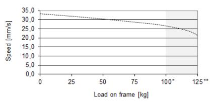
Above curve applies to a centrally placed load and is only valid in respect of duty cycle: 10% by 50% of max. working load or max. 2 min. continuously. Above specifications may vary depending on local temperature, humidity and input voltage.
