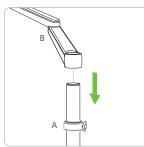
1 Slide the retaining ring (A) onto the column, then insert the double section arm (B) onto upright column.
