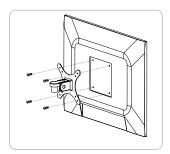
7 Place VESA bracket in position on back of the monitor with lip facing up, attach using 4 screws provided.
