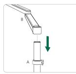
Slide the retaining ring (A) onto the column and set at desired height. Tighten the locking screw using 3mm hex key supplied. Then slide arm (B) onto column.
