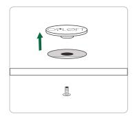
2 Remove disc on Opløft surface by removing the screw from underneath using screw driver. Keep disc and screw in a safe place.
