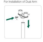
6 Slide the dual arm connector (B) onto the column. Set to desired height and tighten screw (C) using 3mm hex key supplied.
