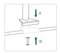
Place the column (A) over hole on Opløft and insert bolt (B) from underneath and securely tighten.
