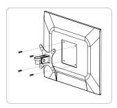
B Place the VESA plate onto the back of the monitor and attach using appropriate screws. Do not over tighten.
