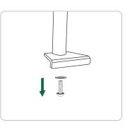
B Remove the base screw from column using the appropriate hex key.
