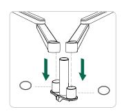
7 Slide the nylon washers onto the dual arm connector then position both arms onto connector.
