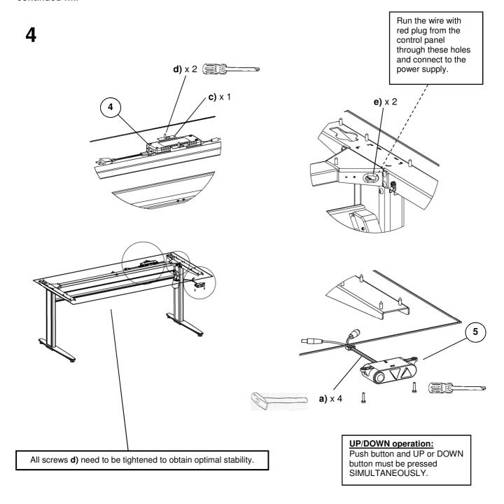
To ensure correct up and down operation of the desk frame it has to be fitted with a tabletop or applied a similar weight. Without a tabletop fitted, the desk frame may not operate in the downward direction.
