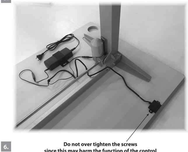
Do not over tighten the screws since this may harm the function of the control
